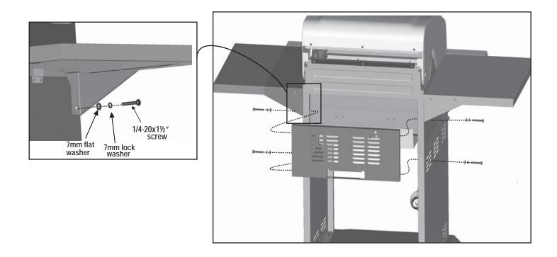
Insert left and right grease tray rails into slots beneath grease tray opening in upper back panel, shown **A**. Attach right and left rails under front brace with two #8x3/8" self-tapping screws, shown **B**.
